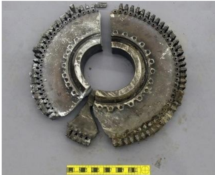
Recovered stage 2 HPT disk pieces (Credits: NTSB)
