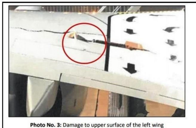
Photo No. 3: Damage to upper surface of the left wing
