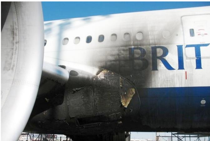
Figure 4. Soot and thermal damage to the right-side fuselage
