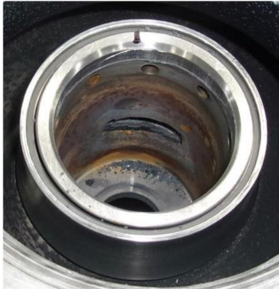
Figure 13: The inside of the turbine end shaft with a hole that had developed at the point of failure of the turbine end journal bearing.
