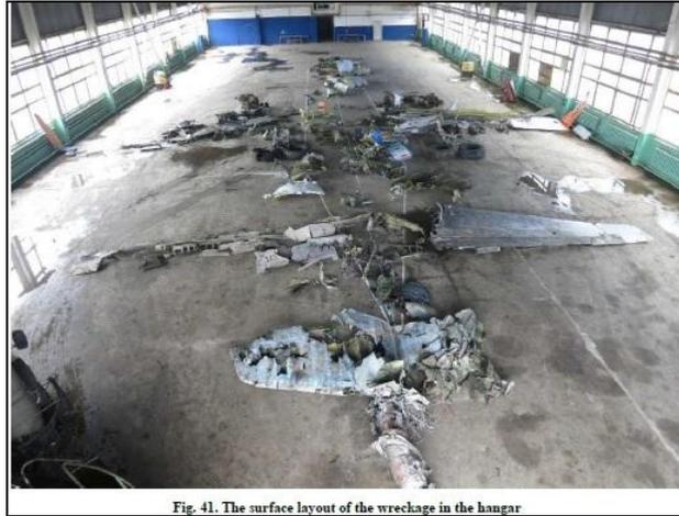
Fig. 41. The surface layout of the wreckage in the hangar
