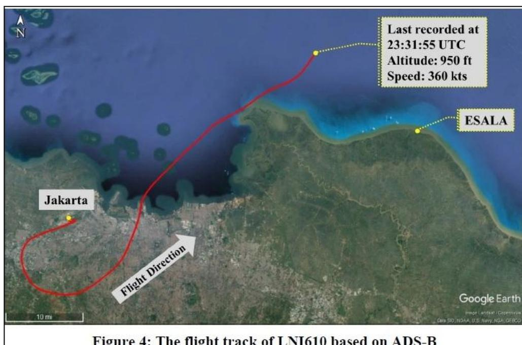
**Figure 4: The flight track of LNI610 based on ADS-B**
